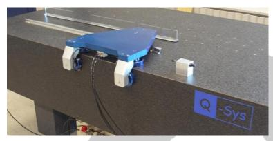
This metrology bench uses vacuum pre-loaded bearings to maintain a constant air gap and to avoid introducing any local stress in the granite bearing surface.
